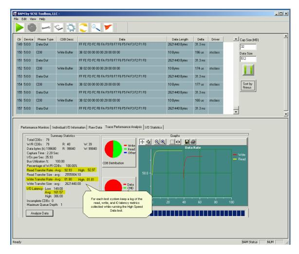
If you notice a change in these numbers, the transfer rates dropping or the IO latency times increasing, thoroughly check and replace any worn cables or connectors.
