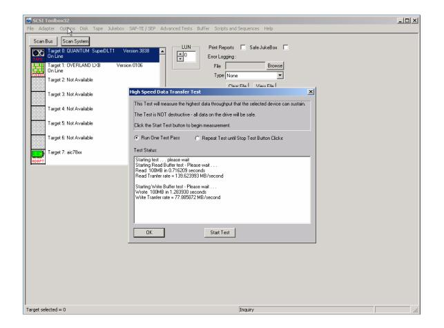
The High Speed Data test transfers data to and from the drive without transferring to the actual drive media. This allows the data transfer speed of the drive and host bus adapter to be determined.
